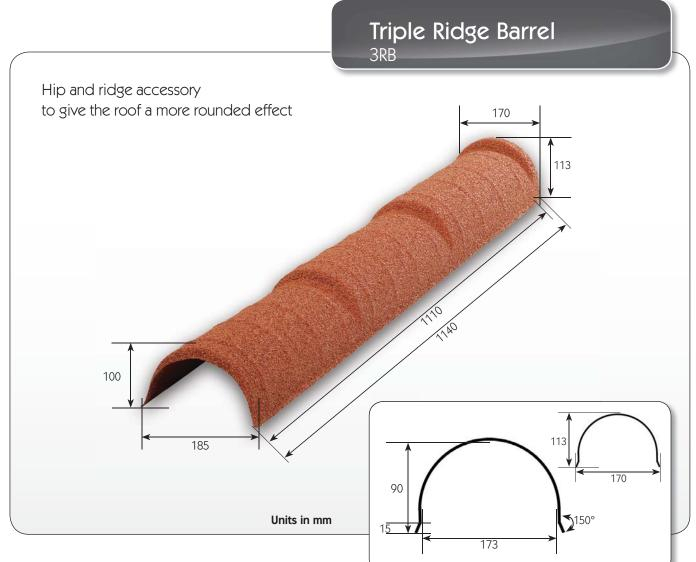
The triple ridge barrel is designed to give your roof a rounded 'finishing' effect. It is pressed from ALUZINC 185 metal and available a wide range of colour in granules, satin, brilliance finish to comply with the rest of the roofing materials.)
