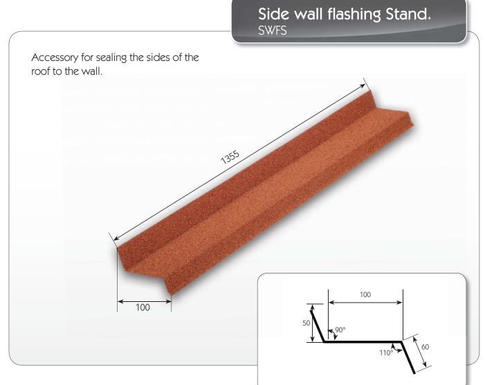
The standard wall flashing is designed to make a nice finish between your roof and the wall that is next to it.
