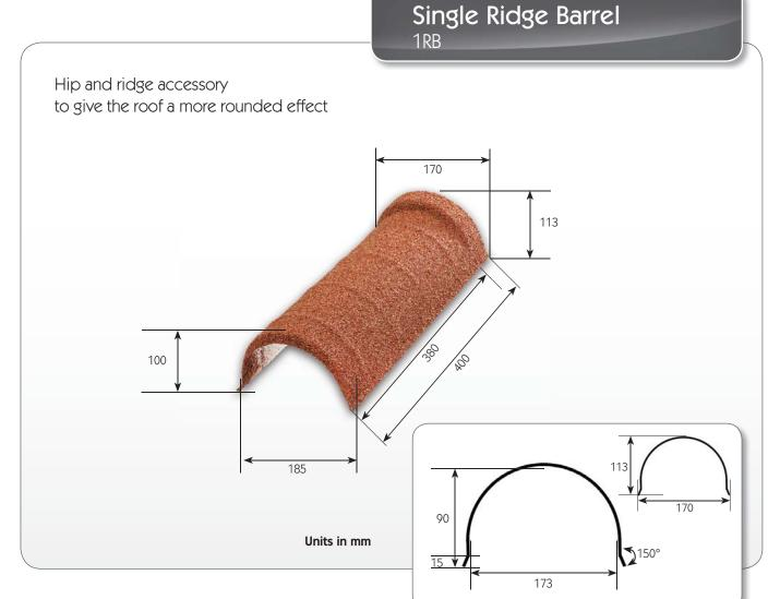
The single ridge barrel is designed to give your roof a rounded 'finishing' effect. It is pressed from ALUZINC 185 metal and available a wide range of colour in granules, satin, brilliance finish to comply with the rest of the roofing materials.
