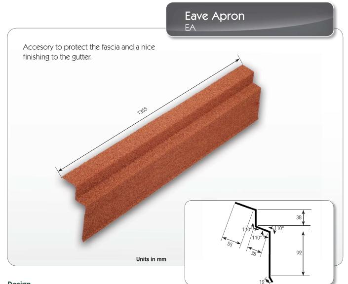
The eave apron is designed to meet a wide range of structural variations for covering the fascia at the bottom course of tile.
